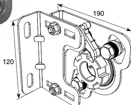
**SPRING SAFETY DEVICE MEDIUM WITH WALL MOUNTING
